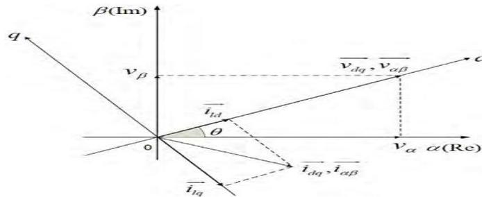
Figure 4.3: Voltage and current components in stationary and rotating synchronous reference frame
