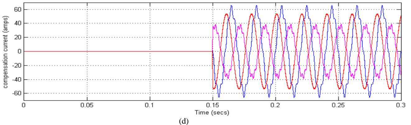
**Fig.5.8. (a) Source voltage (b) Source current (c) Load current (d) Compensated current**
