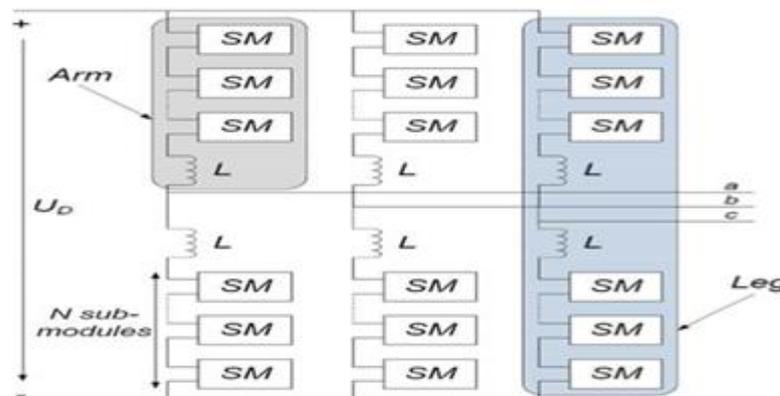
Figure 2.9. Inverter's Leg configuration
