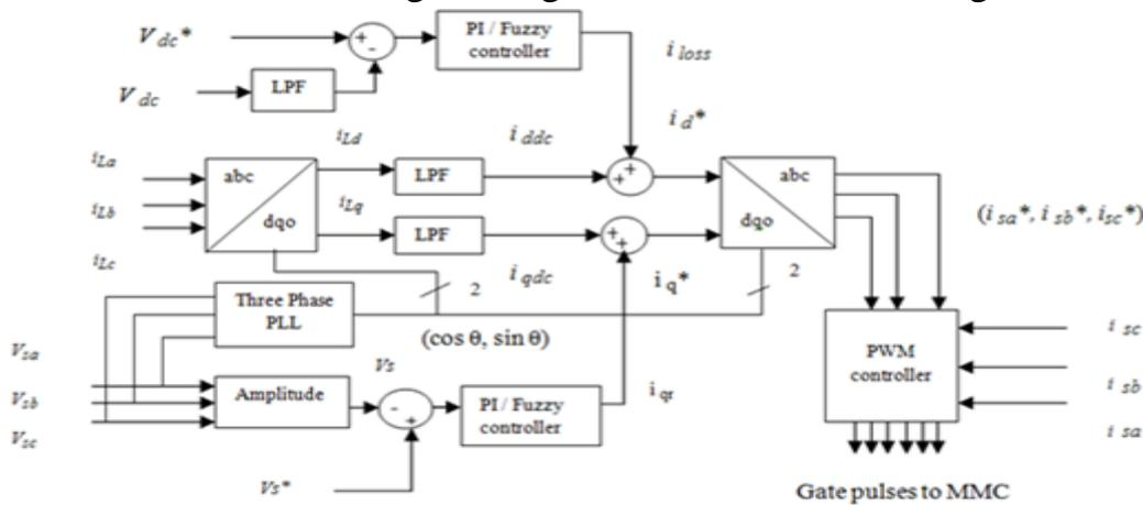
Figure 4.2: General schematic diagram for synchronous reference frame control structure
