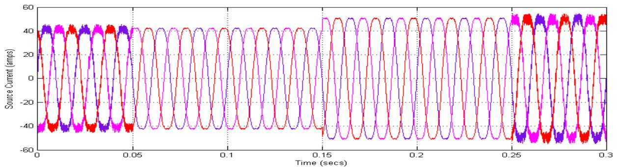
**Figure: 5.5 compensated source current using CHB converter (additional Load)**
