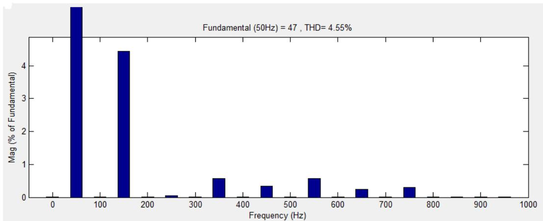
Figure: 5.11 THD of compensated source current using MMC converter
