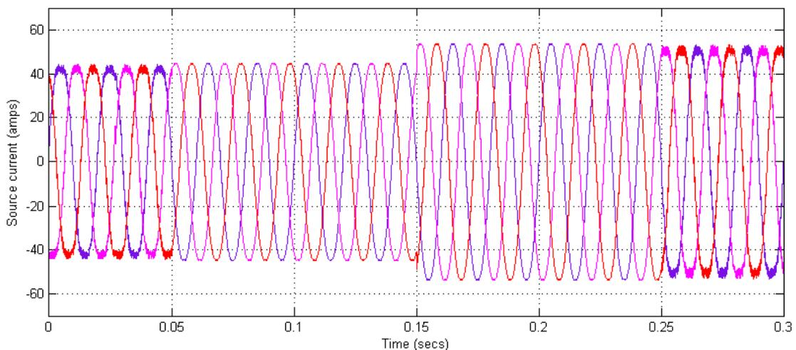
**Figure: 5.9 compensated source current using MMC converter (additional Load)**
