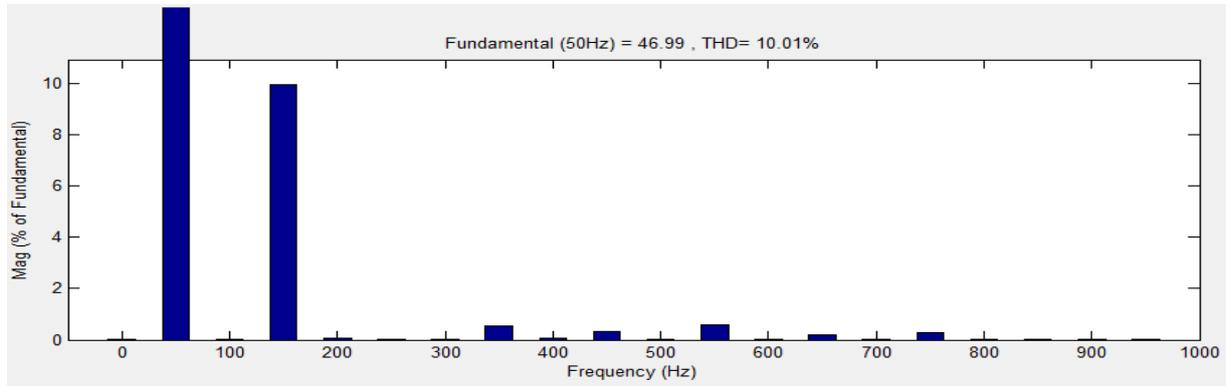
Figure 5.7: THD of compensated Source current using CHB converter
