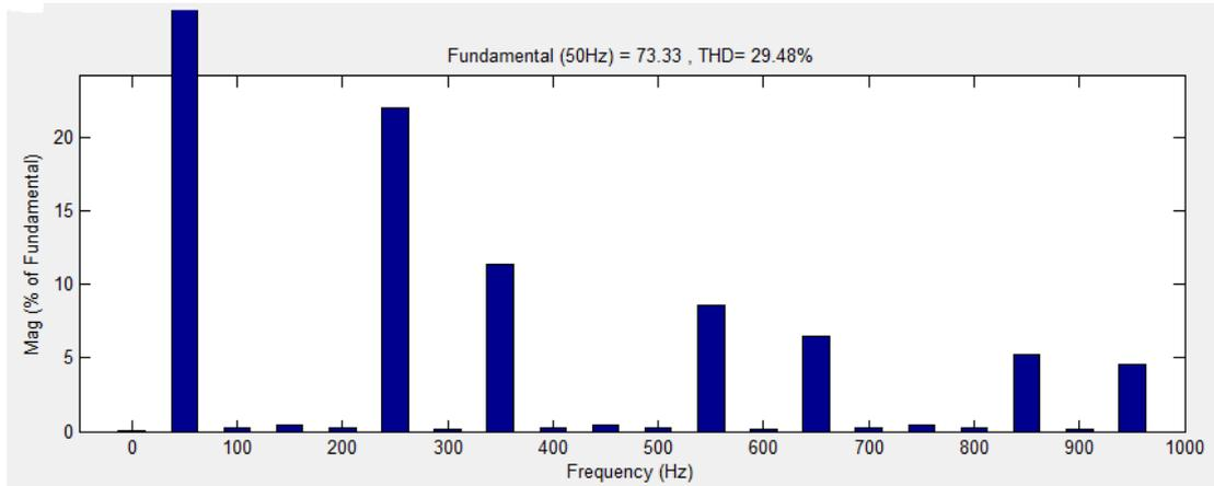
Figure: 5.10 THD of Load Current Spectra
