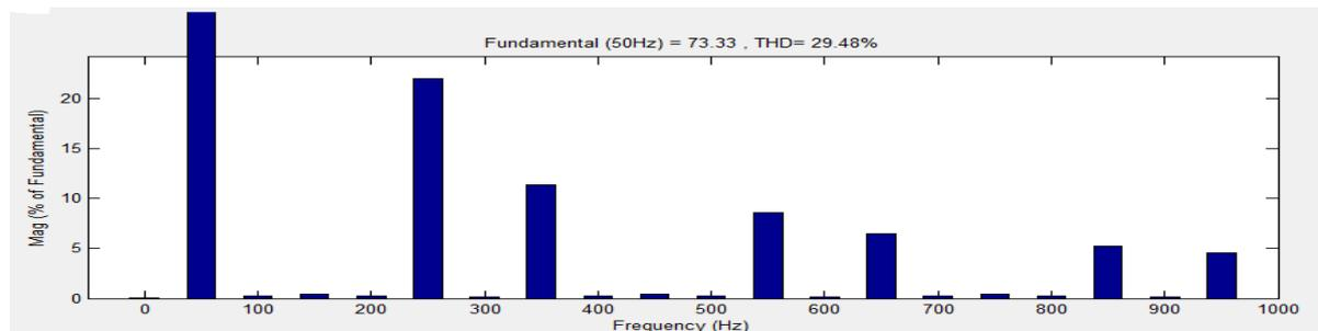
**Figure: 5.6 THD of Load Current Spectra**
